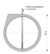
Shut-off damper with blade actuator attached.
