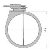
Shut-off damper with manually operation.
