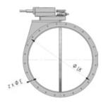
Shut-off damper with manually operation.
