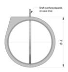
Shut-off damper with blade actuator attached.
